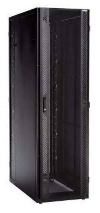
Data center racks have become taller, wider and deeper to accommodate increasing equipment densities. The most popular racks are 42U, 45U or 48U high, 24 inches or 30 inches wide and 42 inches or 48 inches deep. However, these industry standard specifications do not indicate how much usable space is available inside the rack. This is an important consideration given that IT managers are "building up" cabinets to maximize valuable data center space.
